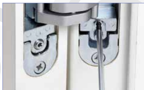
2. Depth adjustment or sealing crushing, door on frame: \pm 1 mm.
