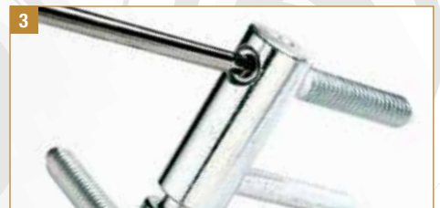
3 By using a "T" wrench it is possible to adjust the height of the pivot, therefore raising the female part. The weight of the door is evenly distributed over all the door-frame hinges thanks to the great sensitivity of the height adjusting device.
