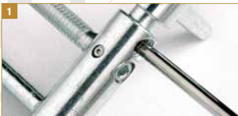
1 By acting on the threaded pin it is possible to quickly fit the hinge using the appropriate hexagonal bit for electrical drill screws and then make the side precision adjustment using the special "T" wrench. The wide, self-threading pitch not only means that assembling time is greatly reduced.
